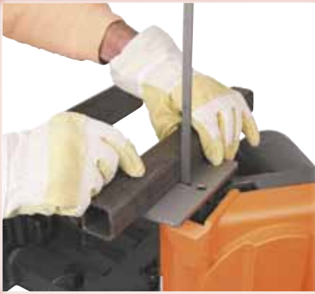
Vertical cutting, here with extended support surface, RBX 120 HV + 180 HV
